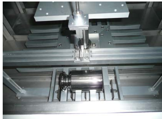
Fig. 11. The suspension strip and weight holder in area C weighing area.
