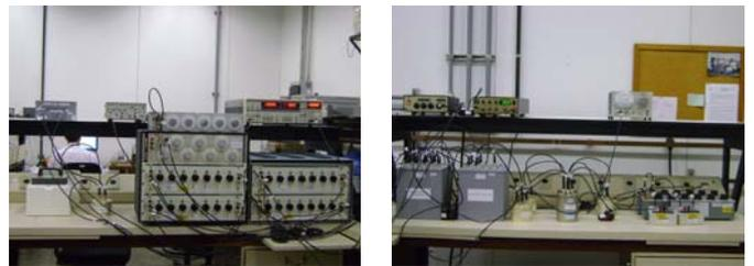
Fig. 2. Four-terminal coaxial bridge.
