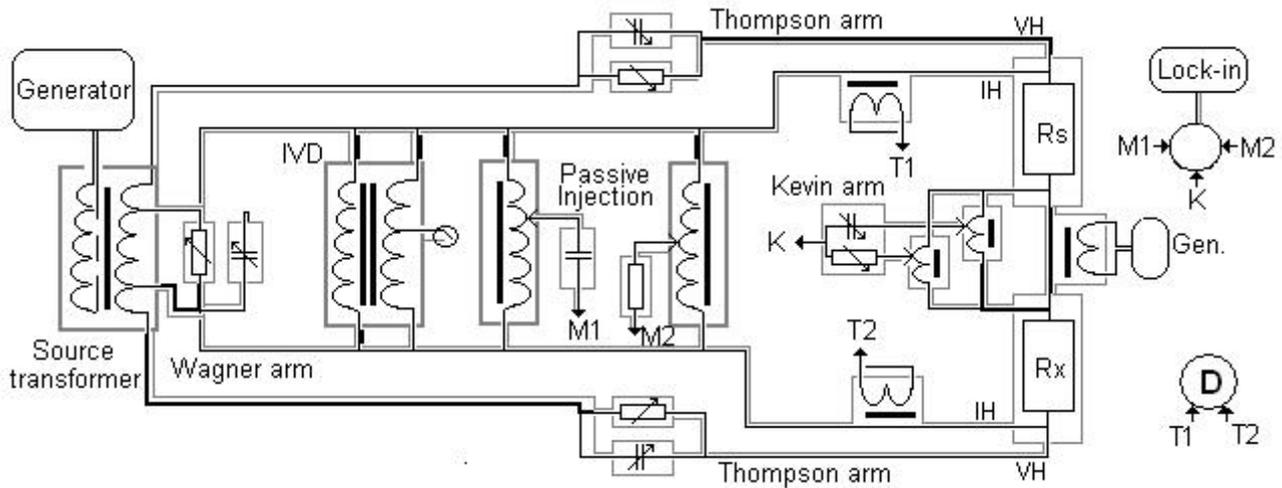
Fig. 1. Four-terminal coaxial bridge.
