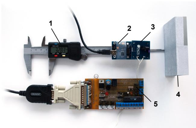
Fig. 4. A short distance sensor system: 1- electronic digital caliper Z22855 Powerfix; 2- LTF EVM motherboard; 3- TAOS LTF EVM TSL245R daughterboard; 4- target object; 5- USTI Evaluation Board.
