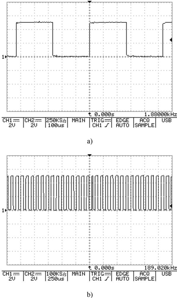
Fig.8 Oscilloscopes at sensor's output at  $f_{x\ min} = \sim 1.83$  kHz (a) and  $f_{x\ max} = \sim 190$  kHz.
