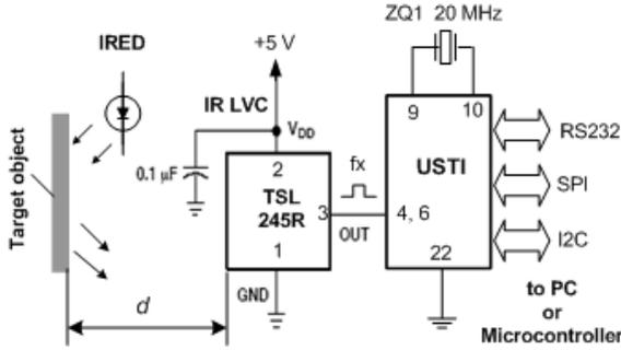
Fig. 1. Short distance measuring system:  $d$  - a distance to be measured; IRED - infrared light source; IR LVC - infrared light-to-frequency converter; USTI- Universal Sensors and Transducers Interface.
