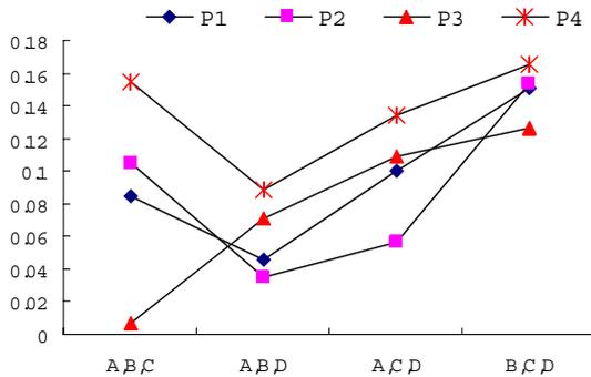
**Figure 7:** Range of position errors caused by the measurements. The vertical axis denotes errors in meters and the horizontal axis shows combination of landmarks used for calculations.
