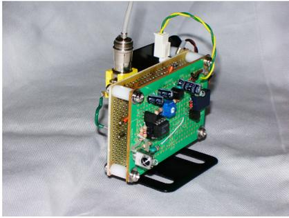
**Figure 3:** RFID tag with a near infrared detector
