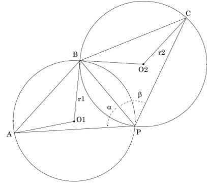
**Figure 2:** Possible robot position lie on an intersection of the two circles.
