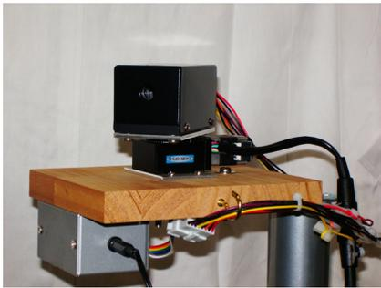
**Figure 4:** Laser light source mounted on the driving gear
