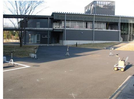
**Figure 5:** Scene of measuring bearing angles to landmarks in a field from the light source on a mobile platform
