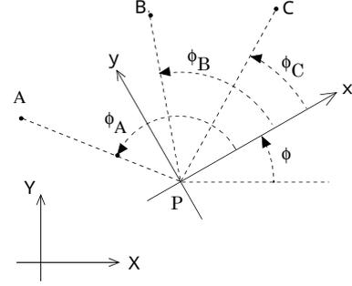
**Figure 1:** Illustration of a planar mobile robot which detects three known landmarks in directions  $\phi_A, \phi_B, \phi_C$ .
