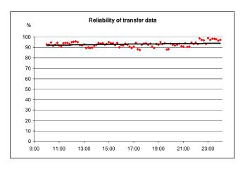
Fig. 6. The reliability of transfer data during a day in a flat, the distance between the transceiver and the receiver 25m
