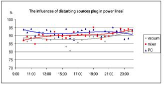
Fig. 7. The influences of disturbing sources in power lines, the distance between the transceiver and the receiver 25m
