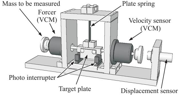
Fig.4 Experimental apparatus
