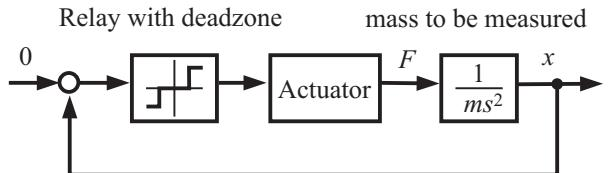
(b) Block diagram of the closed-loop system
