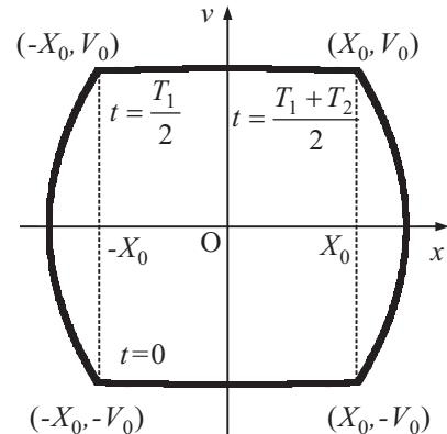
Fig.3 Trajectory of the steady-state response
