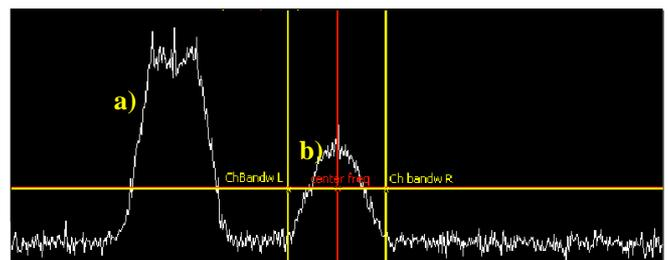
Fig. 5. PSK modulated signal (a) and wideband noise modulated Signal (b) spectra.
