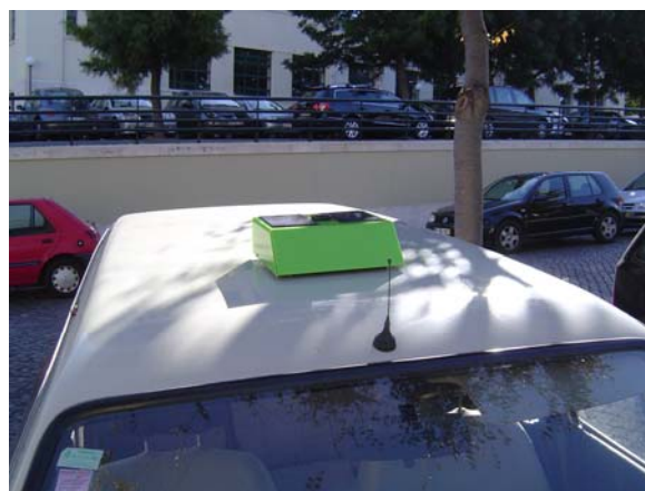
Fig. 1. Photograph of the mobile station prototype mounted on the rooftop of a car.
