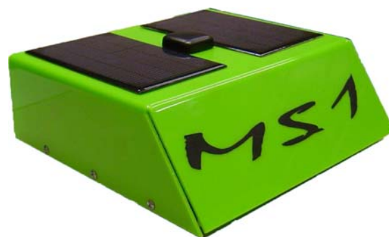
Fig. 2. Outside view of a prototype of the mobile station. On top of the station it is possible to see two solar panels and the GPS receiver antenna.
