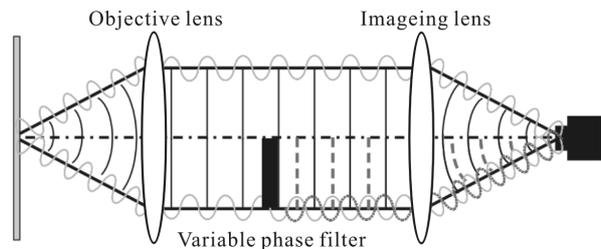
Fig. 2 Imaging-type Fourier spectroscopy method by phase-shift interference between object lights
