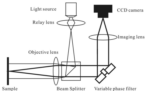
Fig. 5 Structure of the optical system used to measure Three-dimensional near-infrared spectroscopic images
