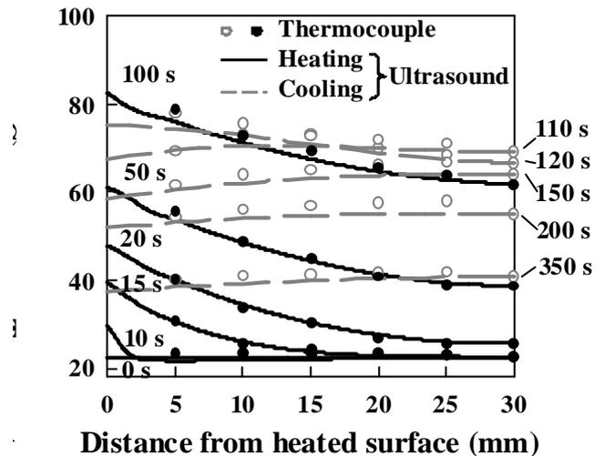
Fig. 5 Variation of temperature distribution in the steel plate with elapsed time, estimated by the ultrasonic method and thermocouples. The numbers in the figure denote the elapsed time after heating starts.
