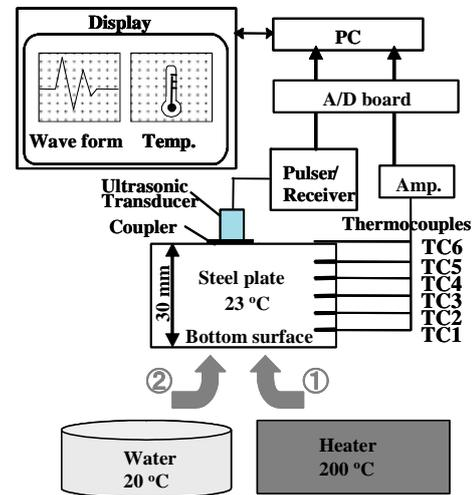
Fig. 2 Schematic of the experimental setup for ultrasonic temperature monitoring.
