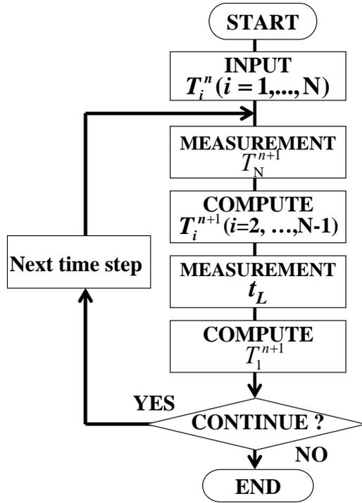
Fig. 1 Flowchart of the inverse analysis for determining the temperature distribution.
