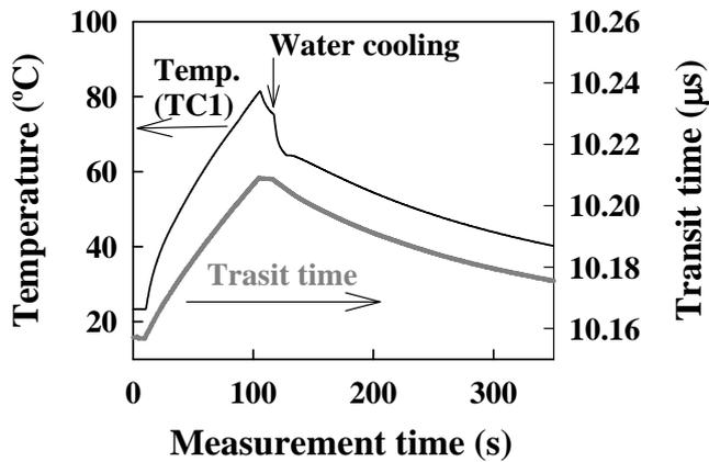
Fig. 4 Variations of the transit time of the ultrasonic wave and temperature in the steel plate during heating and cooling.
