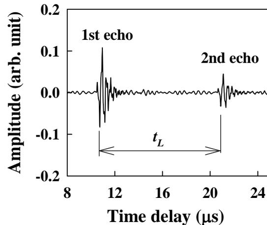
Fig. 3 Ultrasonic echoes reflected from the bottom surface of the steel plate.
