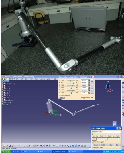
Fig.4. Photo of the real position of CMA and simulated in program Catia v5
