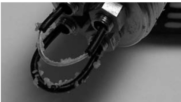
Fig. 8. Photograph of the dusty sensors, contaminated with the deposited crystals of potassium bitartrate.
