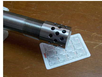
Fig. 4. Photograph showing the support of the fibers with the protection.
