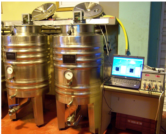
Fig. 7. Photograph of the sensors in the barrels.
