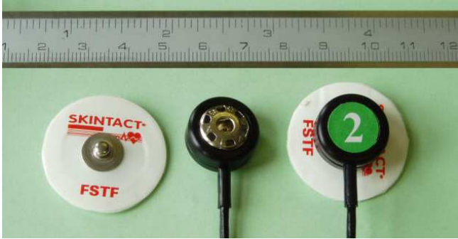
Fig. 9. Active electrodes are composed of quality Ag-AgCl disposable electrodes and active electrode adapter
