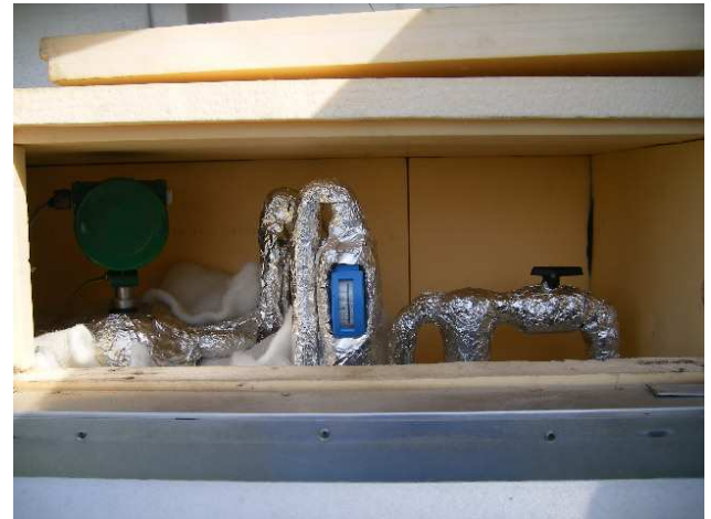
Fig. 7: Level II of insulation.
