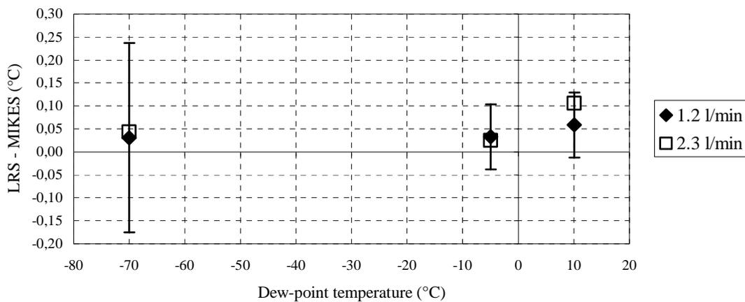
Fig. 2. Difference between the dew-point temperatures determined from the LRS saturator temperature & pressure and the MBW 373 LX indication (applying MIKES calibration results). Error bars show the expanded uncertainty ( $k=2$ ) including uncertainty components related to the hygrometer and the uncertainty of temperature and pressure measurements.
