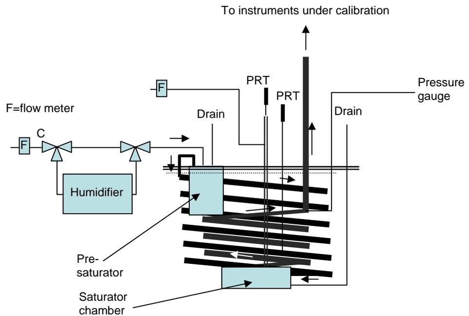
Fig. 1. Schematic diagram of the low-range saturator (LRS).
