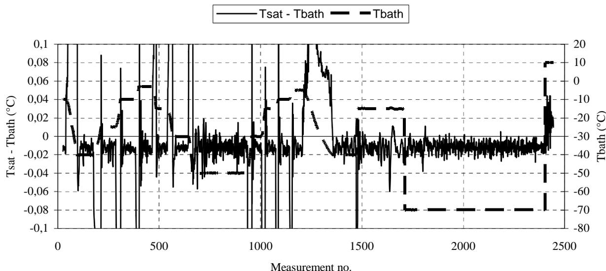
Fig. 3. Difference between the temperatures measured inside the LRS saturator and in the liquid bath close to the saturator, respectively. The corresponding bath temperature is shown with the dashed line. Its scale is shown on the secondary y-axis on the right.
