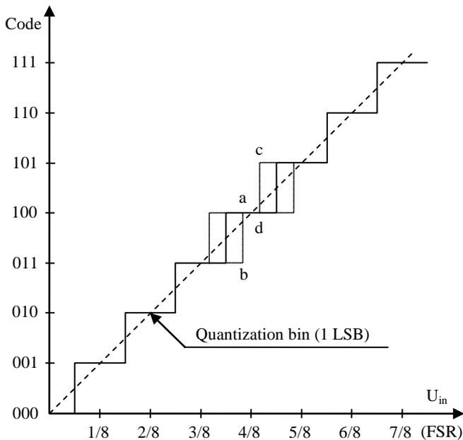
Fig. 2. The transfer characteristic of the ideal 3-bit ADC with  $FSR=8V$ .
