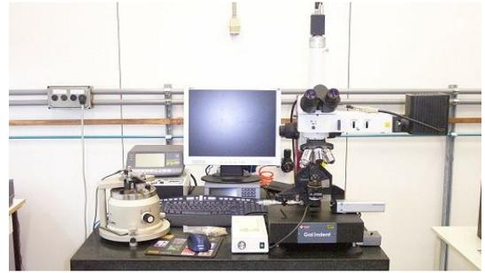
Figure 2 – Primary System of Rockwell and Vickers Diamond Indenters Calibration (Gal-Indent).
