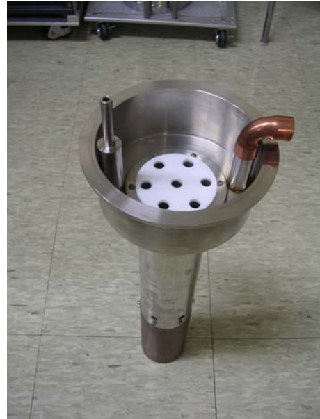
Fig. 5. Photograph of the liquid nitrogen comparison block.
