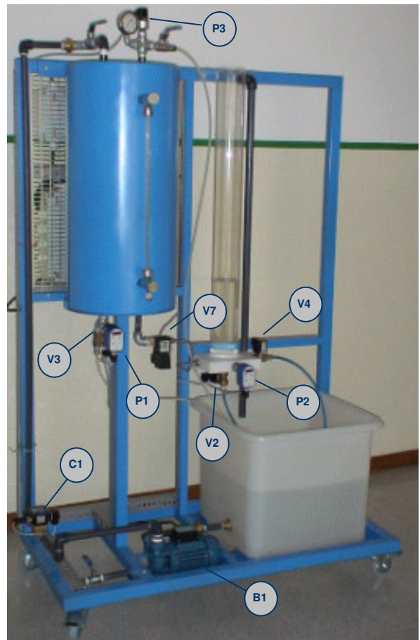
Fig. 2. Experimental set-up of level control system.
