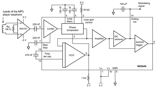
Fig. 3. Circuit diagram of the FM demodulator.
