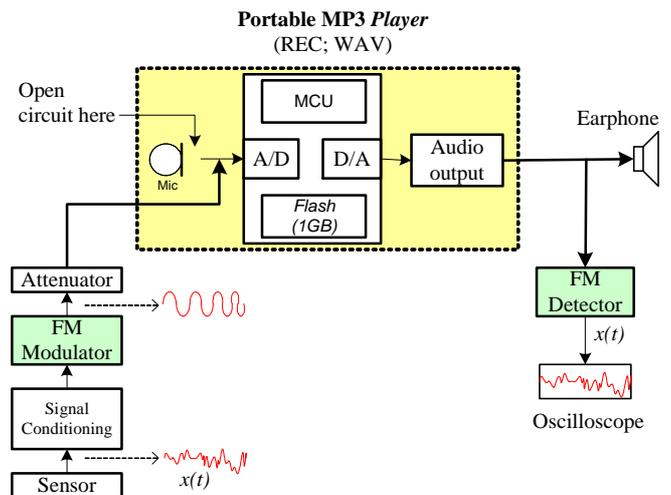
Fig. 1. Block diagram of technique to use MP3 player as a non-audio signal data logger.
