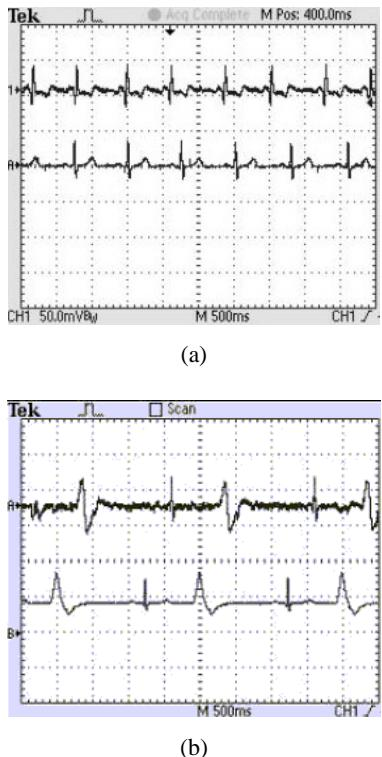
Fig. 6. (a) Patient ECG: (bottom trace) input to FM modulator; (top trace) output of FM detector. (b) Simulated ECG: (bottom trace) input to FM modulator; (top trace) output of FM detector.
