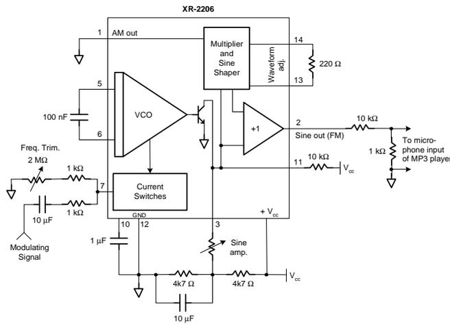
Fig. 2. Circuit diagram of the FM modulator and attenuator.
