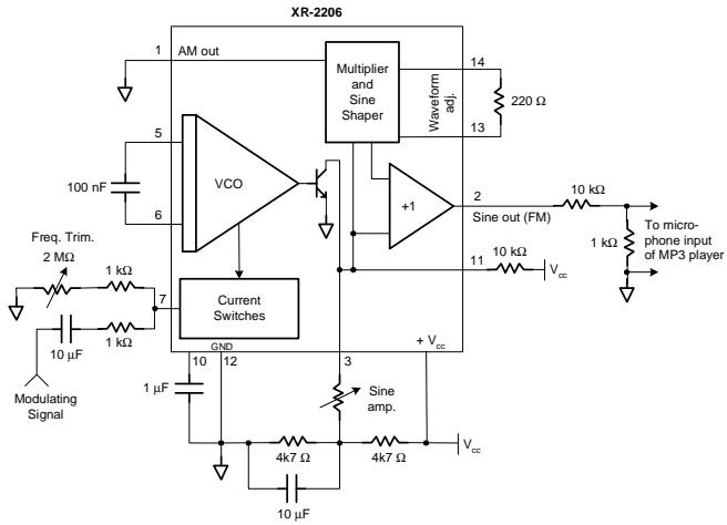
Fig. 2. Circuit diagram of the FM modulator and attenuator.
