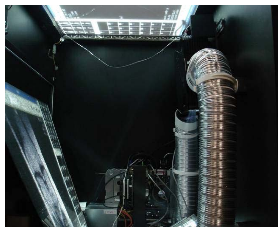
Fig. 4. Internal components of the multi-touch device and the cooling system.
