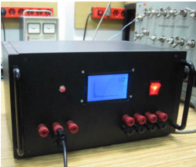
Fig 4. The prototype instrument for Fourier coefficients measurements, with the Fourier spectrum on the LCD display [8].
