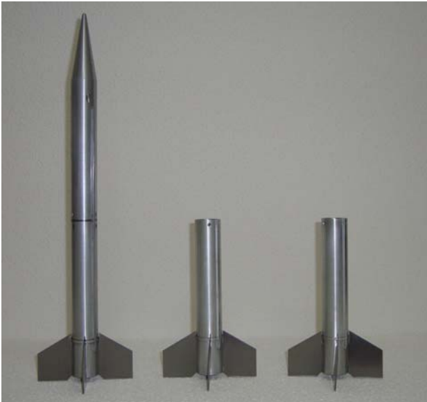
Fig. 3. The second stage Sonda III models. From left to right, fins at 0^\circ , 2.5^\circ and 5^\circ .
