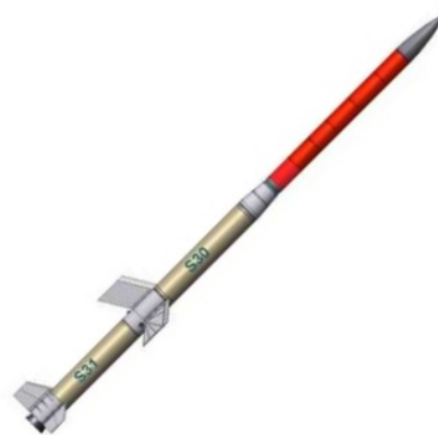
Fig. 1. The VSB-30 two stage suborbital vehicle.
