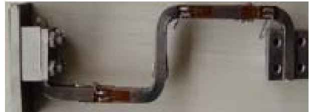
Fig. 4. Detail of strain gauges “S-sensor”
