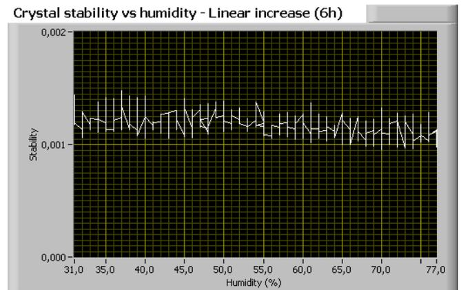
Fig. 11. Crystal frequency offset when humidity is increased from 30% to 77% in 6 hours.
