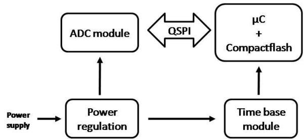
Fig. 3. Acquisition system block diagram
