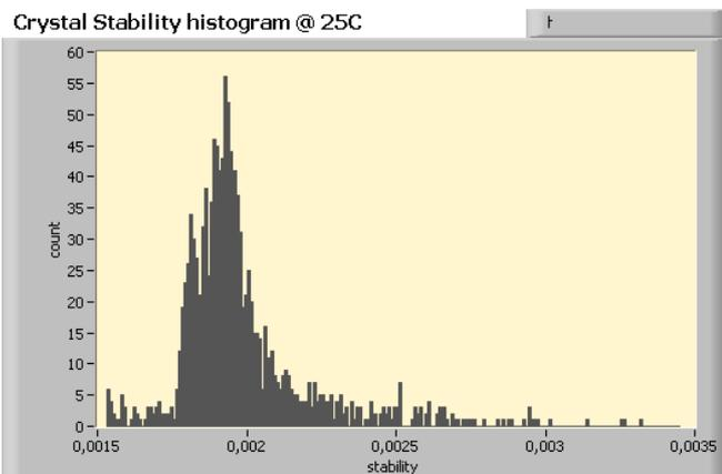
Fig. 9. Crystal frequency offset distribution at 25°C.
