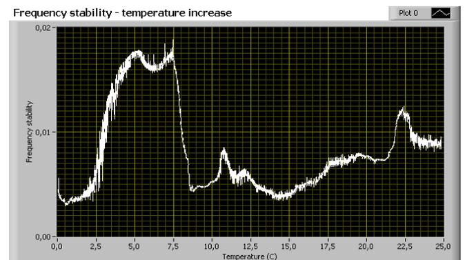
Fig. 6. Crystal frequency offset when temperature is increased from 0°C to 25°C.
