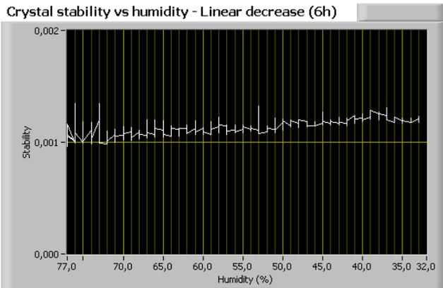
Fig. 12. Crystal frequency offset when humidity is decreased from 77% to 30% in 6 hours.
