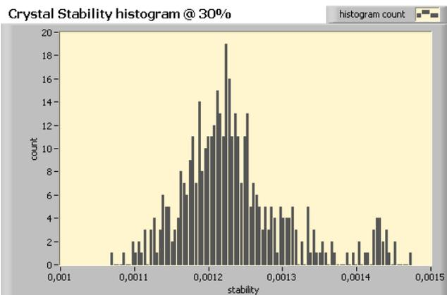
Fig. 13. Crystal frequency offset distribution when the humidity is 30%
