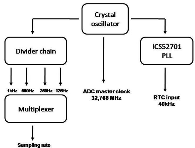
Fig. 4. Time base module block diagram
