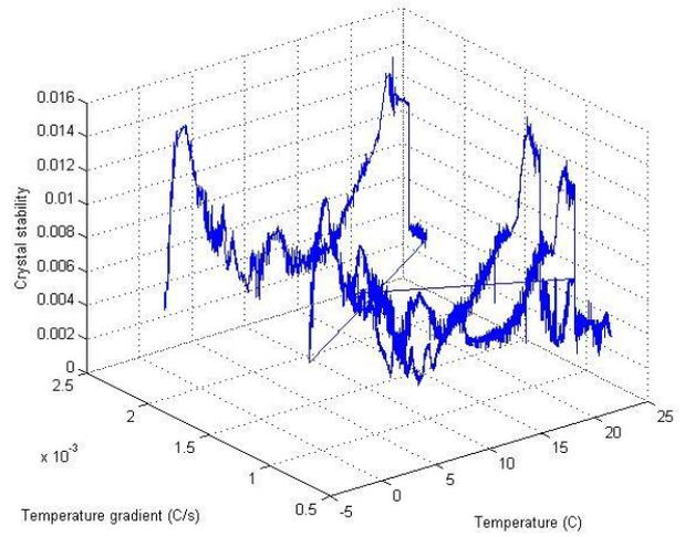
Fig. 10. Effect of temperature gradient on crystal stability when temperature is increased from 0°C to 25°C in 3, 6 and 9 hours.
