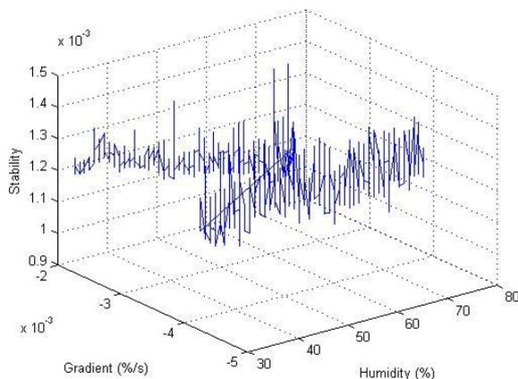
Fig. 14. Effect of humidity gradient on crystal frequency offset when the humidity is decreased from 77% to 30% in 3 and 6 hours. Temperature is kept at 30°C constant.
