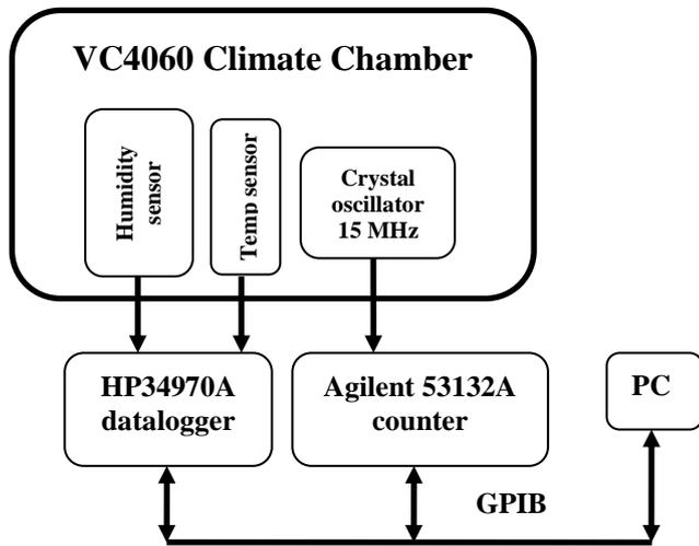
Fig. 5. Measurement system block diagram
