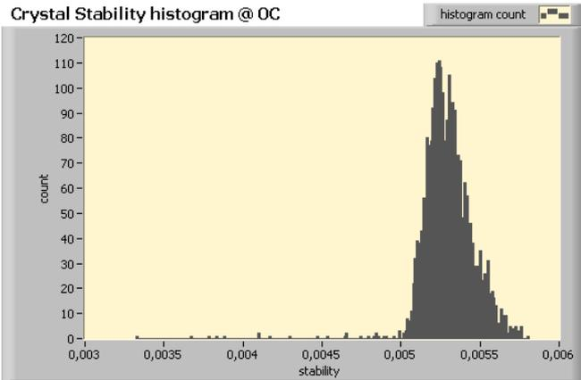
Fig. 8. Crystal frequency offset distribution at 0°C.
