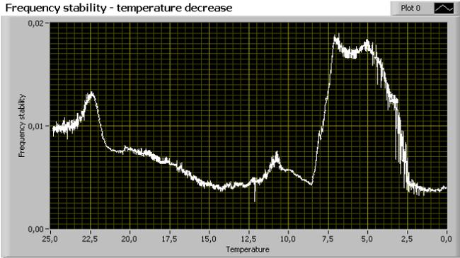
Fig. 7. Crystal frequency offset when temperature is decreased from 25°C to 0°C.
