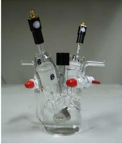
Fig. 1. I.N.Ri.M. flow-through cell
