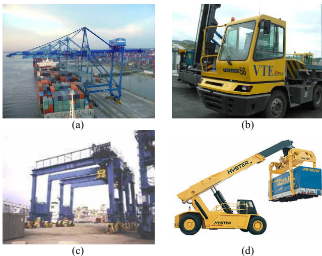
Figure 1 – Container handling vehicles: (a) portainer, (b) tractor, (c) straddle crane, (d) reach stacker.
