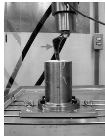
Fig. 1. Picture illustrating a test configuration of the hip femoral steam, according to ASTM F 1440 [5]. The arrow indicates the implant being tested.
