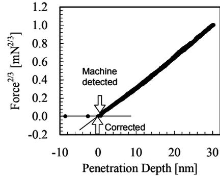
Fig. 3. Modified force-depth curve for sapphire.
