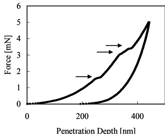
Fig. 1. Typical force-depth curve of low-k film.
