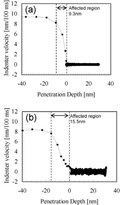
Fig. 2 Typical indenter velocity for Sapphire (a) and low-k film (b).
