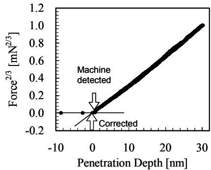
Fig. 3. Modified force-depth curve for sapphire.
