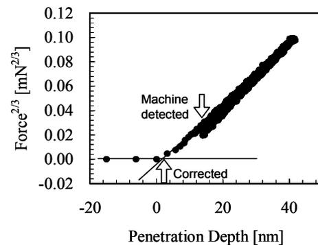
Fig. 4. Modified force-depth curve for low-k film.
