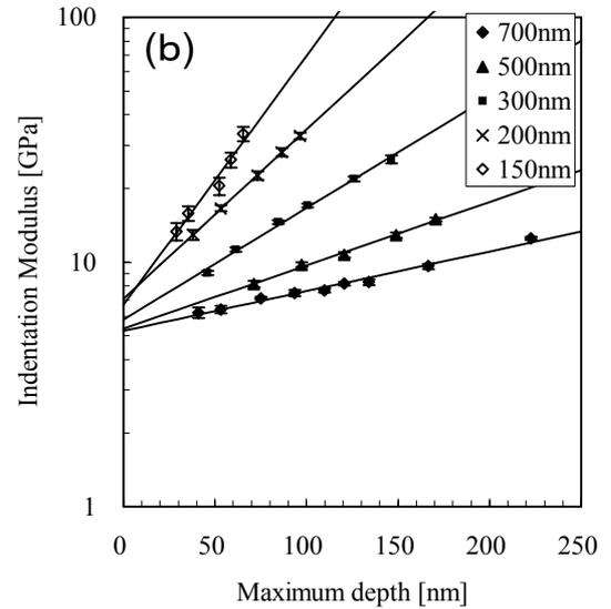
Fig. 6. Indentation modulus obtained with proposed contact point correction.
