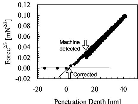
Fig. 4. Modified force-depth curve for low-k film.
