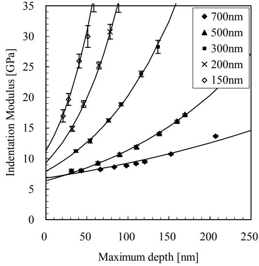
Fig. 5. Indentation modulus obtained by using Machine detected zero point.
