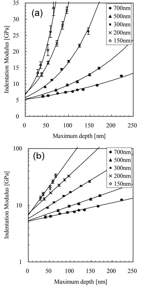
Fig. 6. Indentation modulus obtained with proposed contact point correction.
