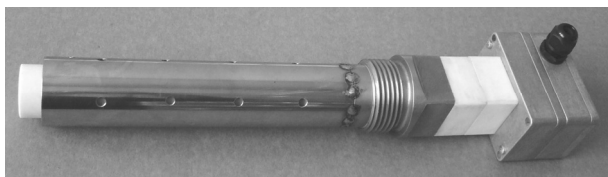
Fig. 7. Sensor for on-line measurement of water content.
