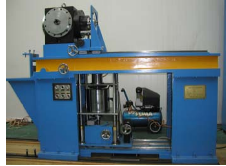
Fig5: 100N·m negative step dynamic torque standard machine
