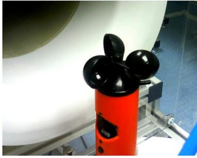
Fig. 12. Verification velocity blockage effects by using cup anemometer.
