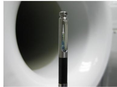
Fig. 10. Verification of velocity blockage effects using an anemometer
