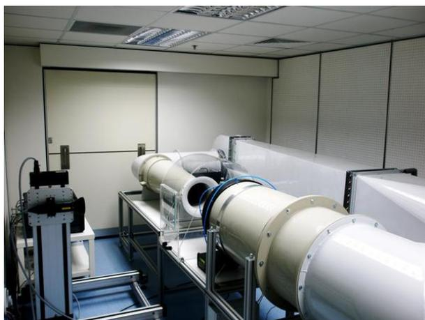
Fig. 1. NMC's primary air velocity standard
