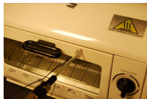
Fig. 5. The position of the probe during measurement horizontally and vertically on the oven
