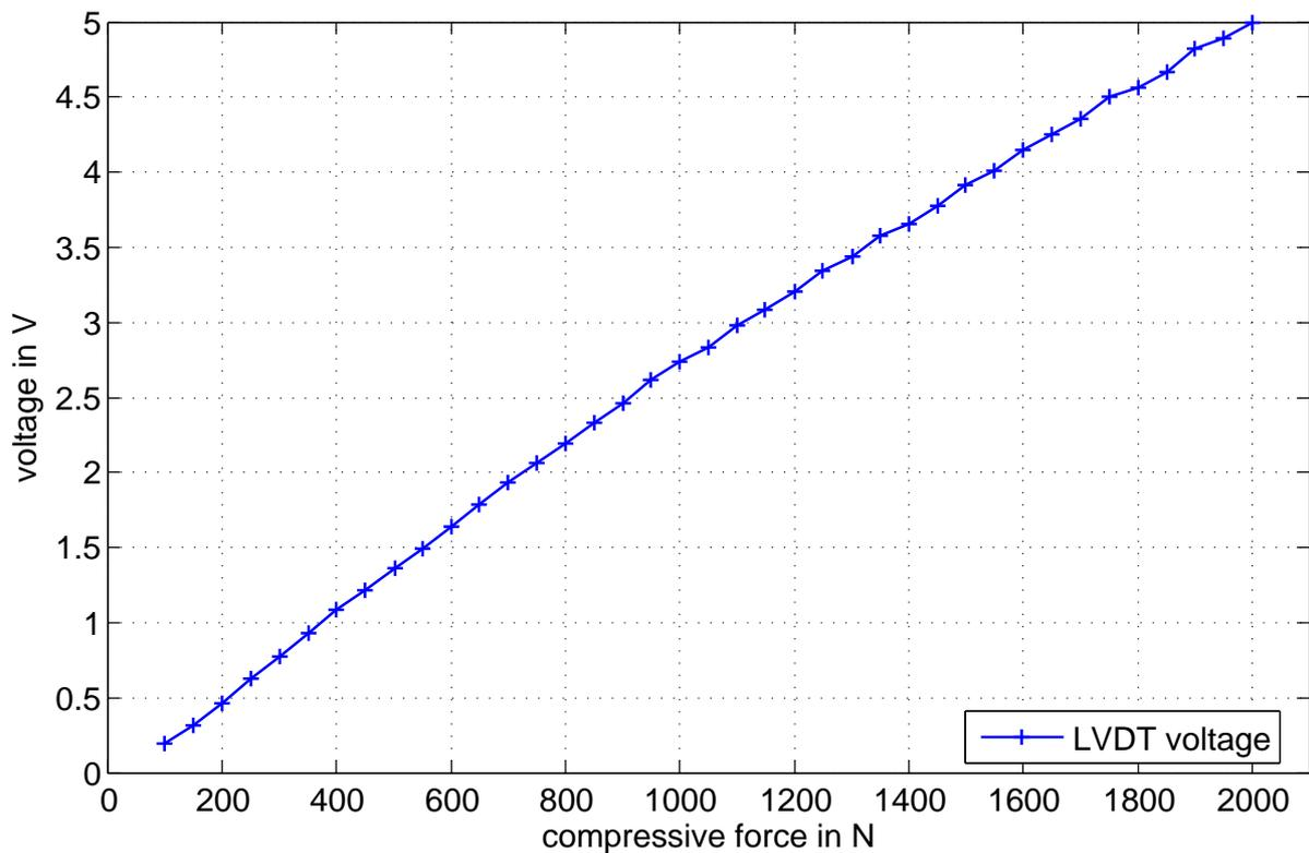
Fig. 5. Output voltage of the LVDT chip vs. the applied mechanical load with quasi-static compressive force steps from 100 N to 2000 N.
