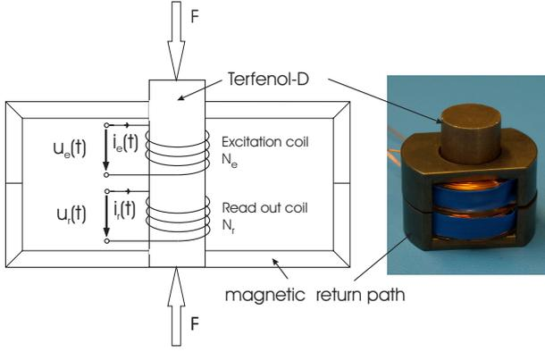
Fig. 1. Schematic model of the sensor with the described return path on the left side and a photo of the prototype on the right side.
