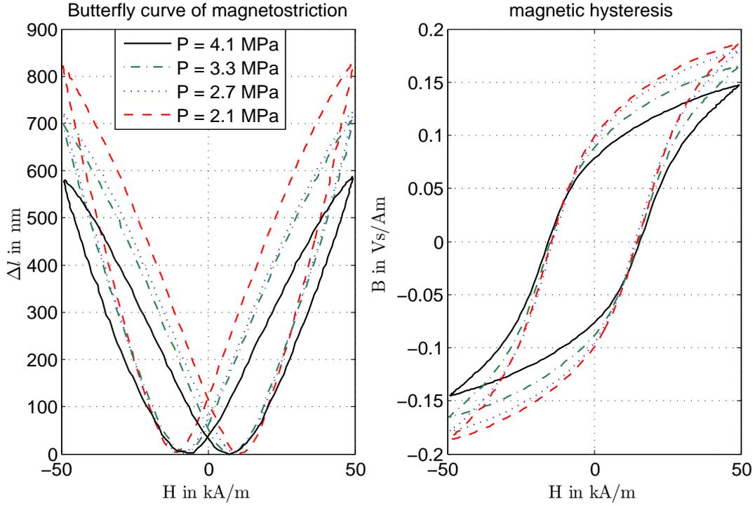
Fig. 2. The left diagram shows the butterfly-curve of the magnetostriction and the right diagram shows the magnetic hysteresis of the sensor material Terfenol-D both with different applied prestresses. The legend of the left diagram describes different prestresses of the curves of both diagrams.
