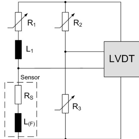
Fig. 4. Assembly of the sensor electronic, which is connected to an AC-bridge. The bridge signal is demodulated and amplified by the LVDT chip of Analog Devices Inc. The LVDT chip delivers an analog output signal, that is proportional to the applied mechanical load.
