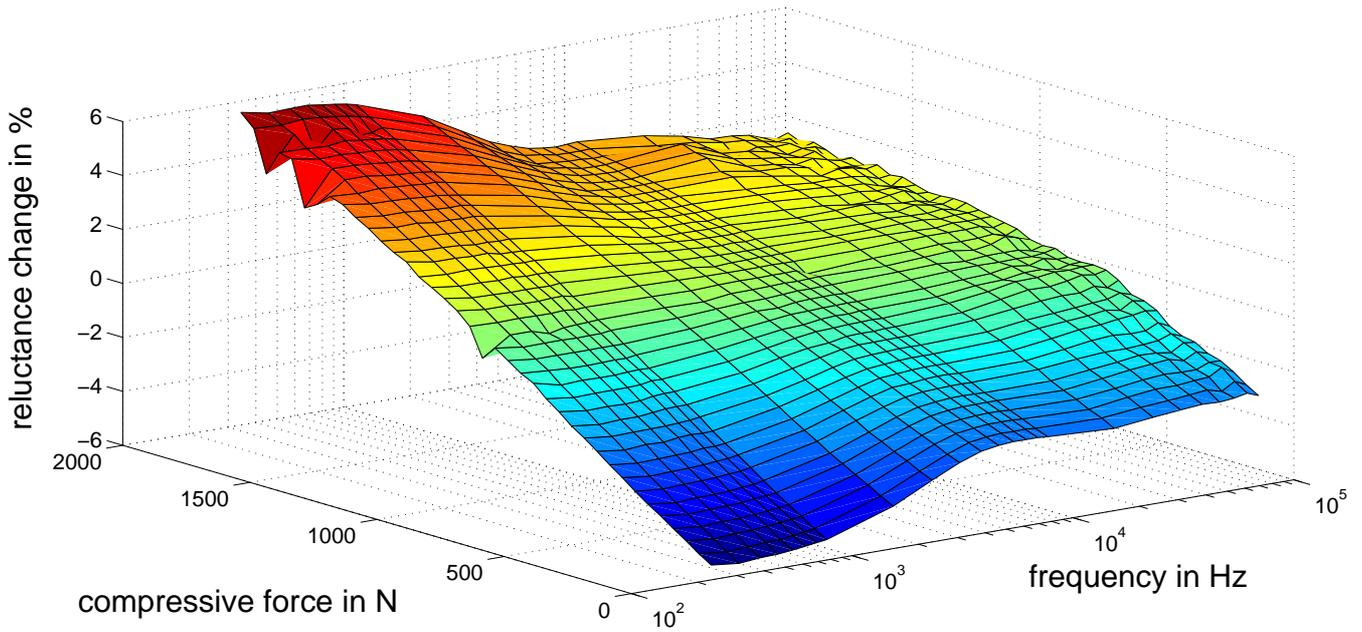
Fig. 3. Relative magnetic resistance change of the set-up (see Fig. 1) vs. applied compressive force and excitation frequency.
