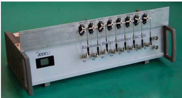
Fig. 3. Manipulator unit on top of RBC100.
