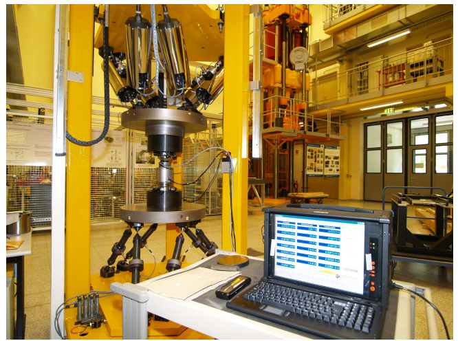
Figure 3. Force vector sensor in multi-component calibration machine
