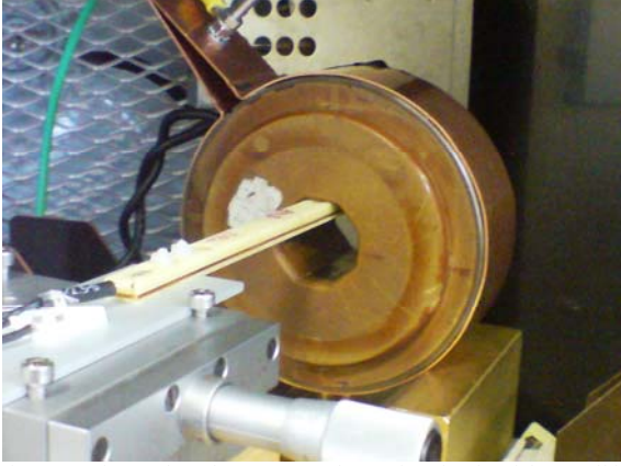
Figure 1: The quadrupole magnet on the test bench. The pick-up coil is mounted facing one of the four poles (embedded inside the insulation, hence not visible) to maximize flux linkage. The copper foil bracket fastened at the outside of the magnet is used to ground the iron yoke, both for safety and for signal integrity reasons.
