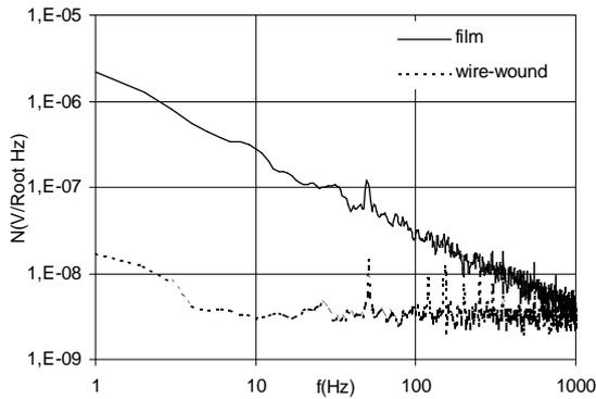
Fig. 7. Noise at the terminals of resistor
