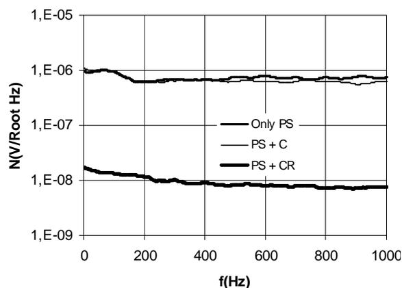
Fig. 3. Signal noise at the output of the DC power source with filters.
