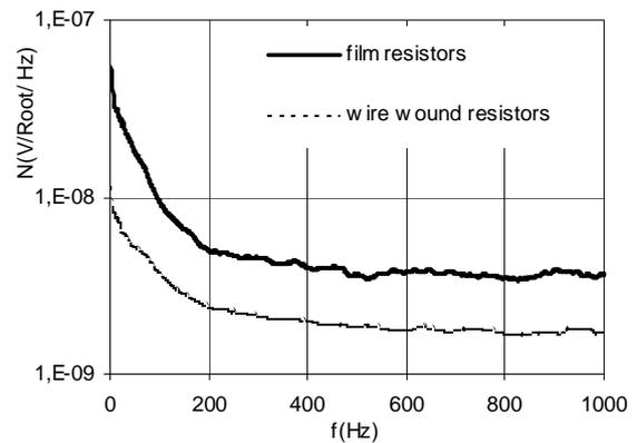
Fig. 9. The noise voltage spectral density of the experimental DC power source
