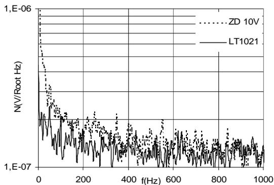
Fig. 4. Signal noise at the output of the reference voltage source and Zener diode stabilizer.
