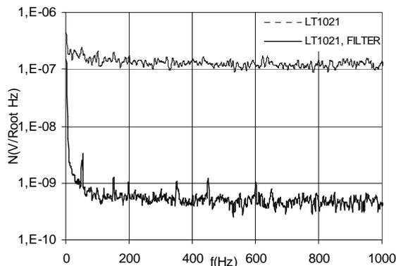
Fig. 5. Signal noise at the output of the reference voltage source and reference voltage source with filter.
