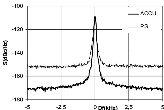
Fig. 1 The noise levels of RF signal generator supplied from accumulator or of laboratory power supply
