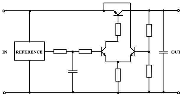
Fig. 8. Discrete transistor DC power source
