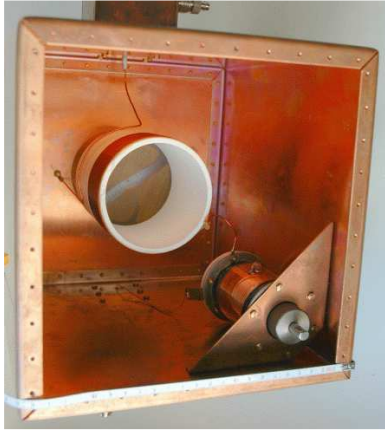
Fig. 9. Input resonant circuit of the filter
