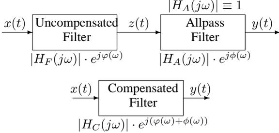
Fig. 1. General scheme of the group delay compensation process.
