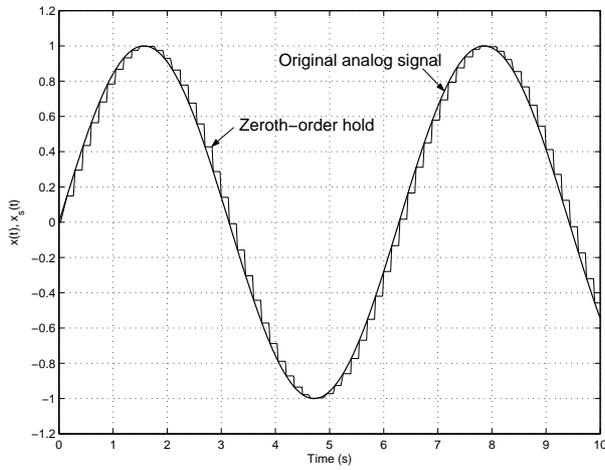
Fig. 4. Original analog signal and its zeroth-order hold equivalent.
