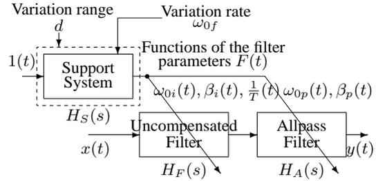
Fig. 2. Block diagram of the proposed parameter-varying filter.
