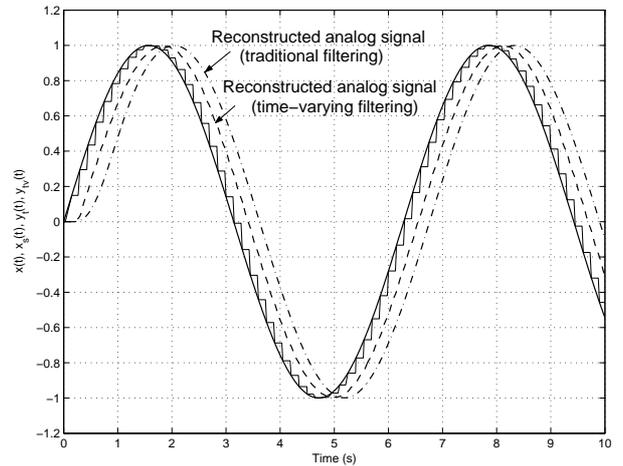
Fig. 8. Simulation results of the parameter-varying filter and the linear time-invariant filter used in the reconstruction of the signal shown in Fig. 4.
