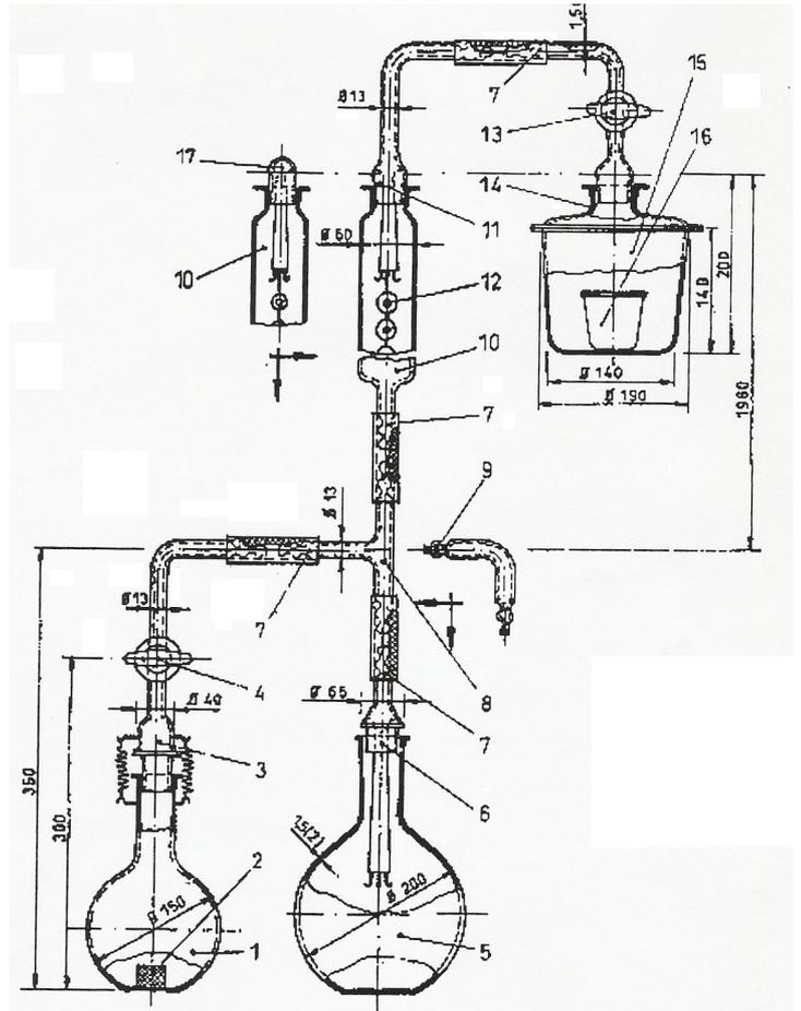
Fig.1. Experimental device for track detectors calibration with <sup>226</sup>Ra-<sup>222</sup>Rn source
