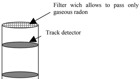
Fig. 2. Alpha monitoring device
