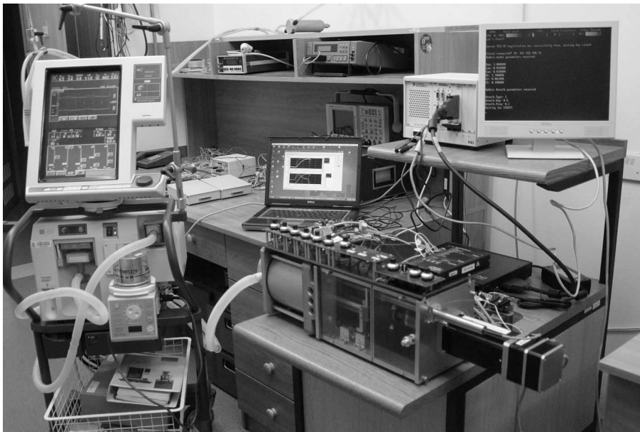
Fig. 8. Laboratory set-up of the hybrid model of lungs
