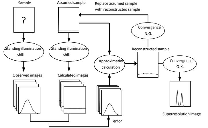
Fig. 2. Block diagram of the super-resolution post-processing
