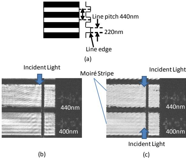
Fig. 14. (a) Schematic diagram of an L&S pattern
