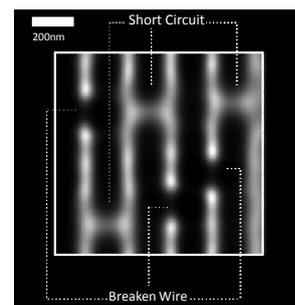
Fig. 9. The 2D super-resolution image obtained by simulation
