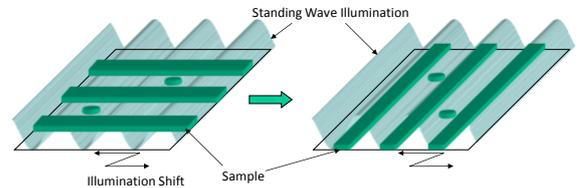
Fig. 4. 2-direction shift of standing wave illumination
