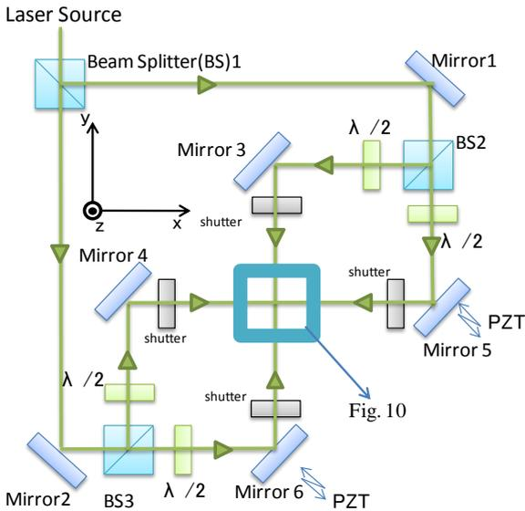
Fig. 10. Schematic diagram of optical system of 4 incident light directions (top view)
