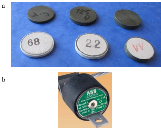
Fig. 2. Varistor specimens: a – ZnO structures after being fired (top row) and with a metalized contacts (bottom row); left – 280 V, middle – 440 V, right – 660 V; b - surge arrester with ZnO varistor
