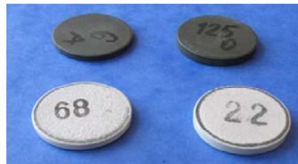
Fig. 1. Tested varistors for working voltage 280 V: ZnO structure after being fired in a stove - top row, with the metal contacts - bottom row
