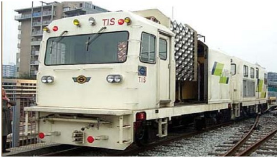
(a) Inspection system of the tunnel lining using an Infrared camera and CCD cameras(Teito Rapid Transport Authority, Japan).
