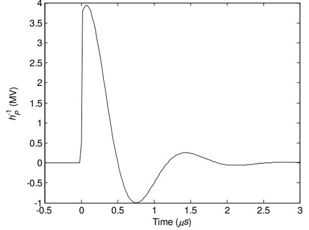
Fig. 3. Simulated impulse response of the estimator  $h_p^{-1}(t)$ .
