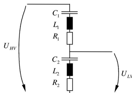
Fig. 1. Equivalent simplified circuit of a voltage divider.
