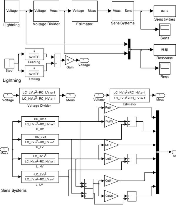
Fig. 2. Simulink model for estimation and generation of dynamic model sensitivity signals. The relative parameters are defined by  $X_q \equiv X_q / X_{HV}$ , where  $X = \{R, L, C\}$ ,  $q = \{1, 2\}$  and  $X_{HV}$  the total for the HV circuit. The RC and LC constants for the HV/LV circuits are labelled RC\_HV/RC\_LV and LC\_HV/LC\_LV, respectively.
