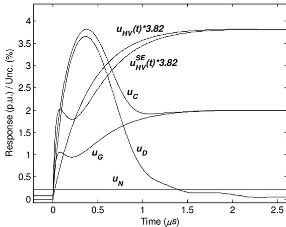
Fig. 5. The leading part of normalized lightning  $u_{HV}$  and related static estimate  $u_{HV}^{SE}$  (both rescaled), and the combined measurement uncertainty  $u_C$  built of  $u_G, u_M, u_N$ .
