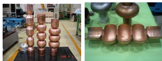
Fig. 3. Seamless three-cell cavities made by necking and hydroforming (test modules made of copper).
