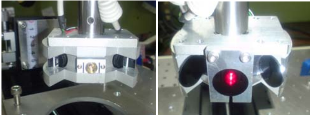
Fig. 14. Measuring Head (Left: bare, Right: with ND filter and light shielding cover).
