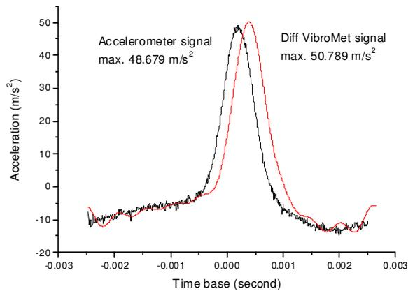
Fig. 6. Compare the output peak shock value derived from laser Doppler vibrometer and accelerometer ( $50 \text{ m/s}^2$ ).
