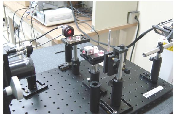
Fig. 8. The interferometer components.
