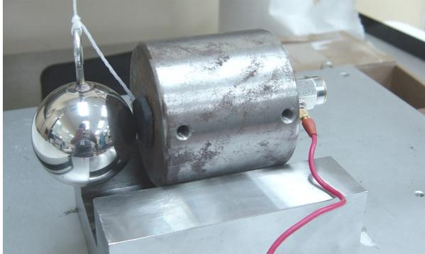
Fig. 2. Simple shock pendulum.
