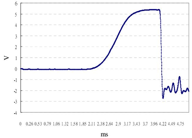
Fig. 5. The output signal from laser Doppler vibrometer.
