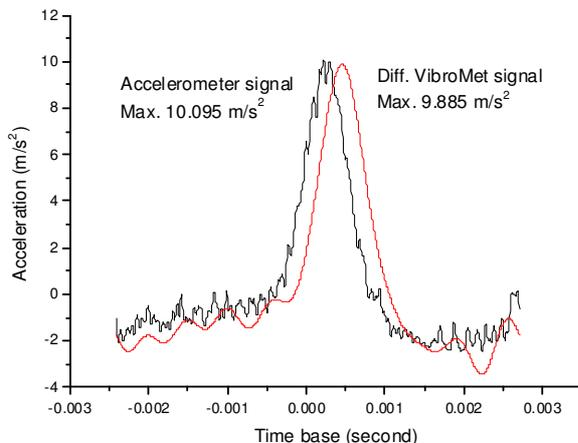
Fig. 7. Compare the peak shock value derived from laser Doppler vibrometer and accelerometer ( $10 \text{ m/s}^2$ ).
