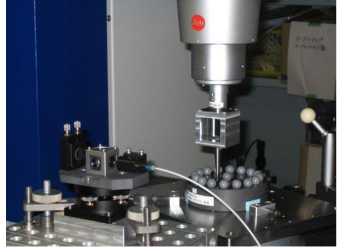
Fig. 9. Photo of the scene of the length calibration using a CMM with an interferometer
