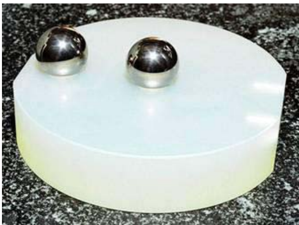
Fig. 2. Photo of the double ball artifact (DBA)
